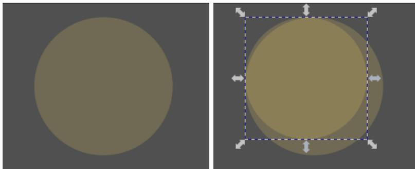
Start with a simple circle, 85mm in diameter. Duplicate it, reduce to 75mm diameter. Center them using alignment tools, and change the smaller circle to green (our cut layer).
