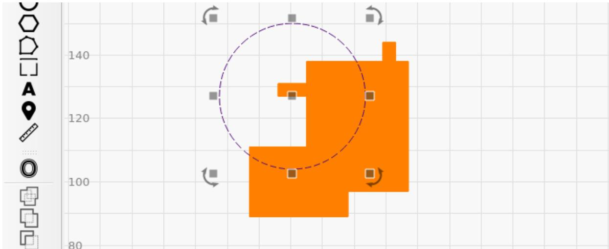
Note that this needs to be done on a new layer. And in Lightburn there is no clipping path - instead we perform a boolean subtraction, specifically an intersection.
