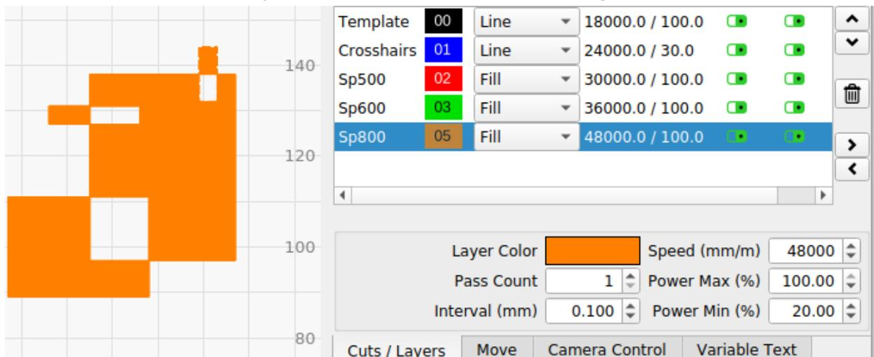
You will notice that anywhere the fills overlap, a subtraction is automatically created. This can cause some very unexpected problems if the source of our design is a separate tool like Inkscape or Illustrator.
