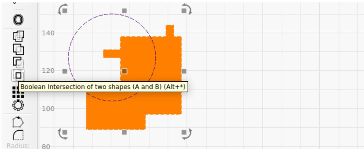
The result is a clipped vector - but note that this clip is destructive - there is no way to un-apply it other than to undo.
