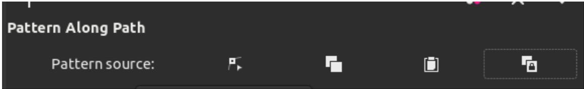
To ensure that the teeth of the saw blade form a complete circle with no gaps, you can use the “Repeated, Stretched” option:
