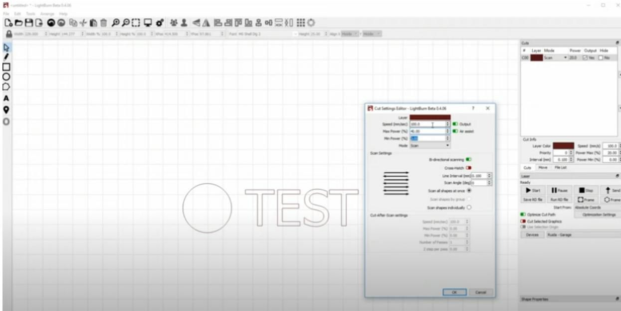
Another factor to know about is something called “interval”. This is how far apart the lines composing the fill are placed. The interval is something that can be modified and controlled.
