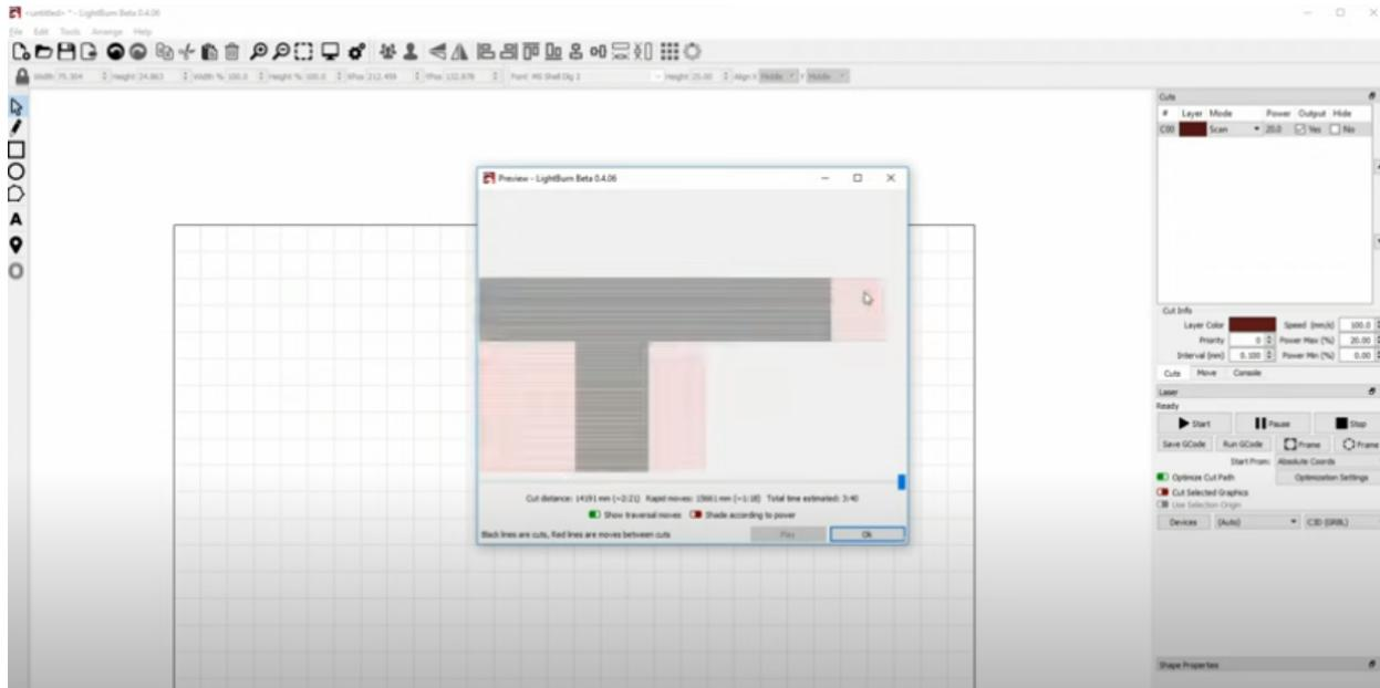
Traversal lines show the overscan in place around the text.
