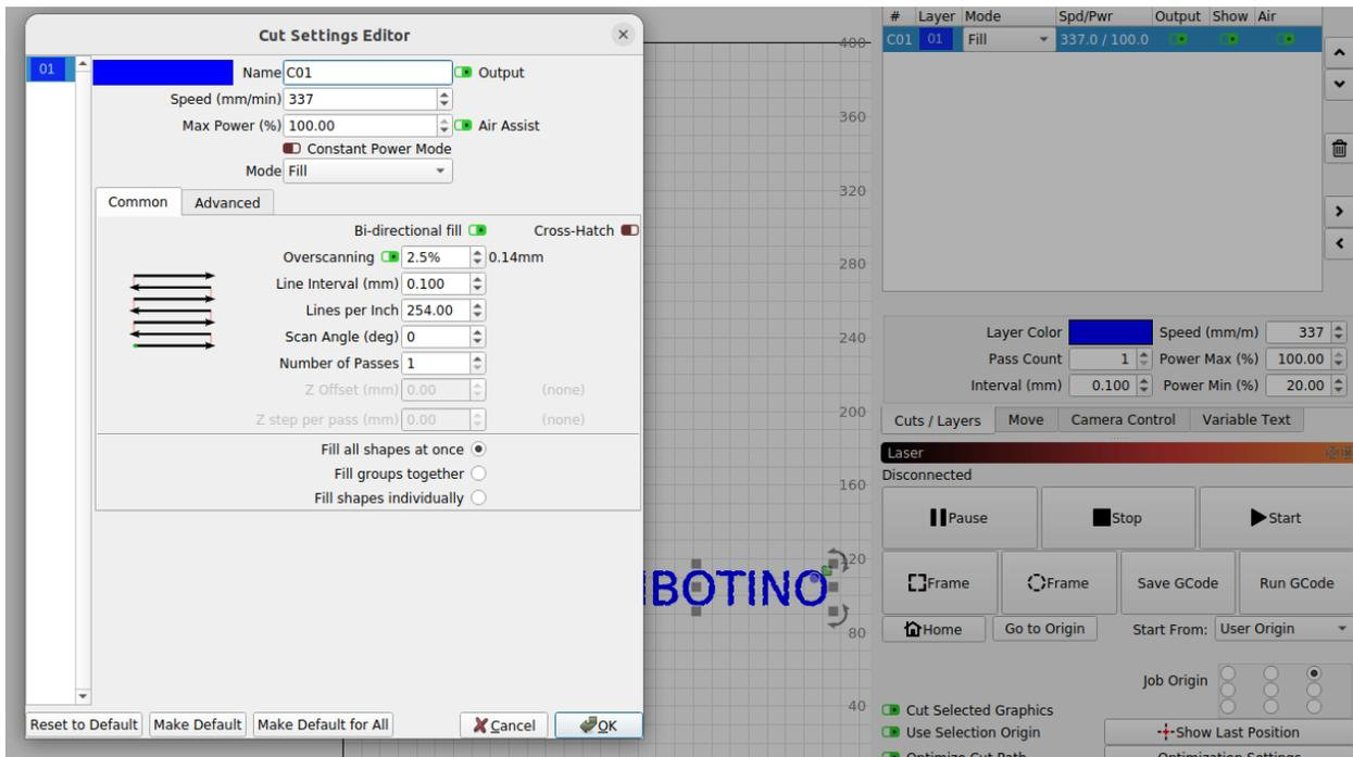
Note in the image above the option “Fill all shapes at once” is selected. This will cause the raster line to traverse the entire line of text in each pass. This can be seen by looking at the preview window.
