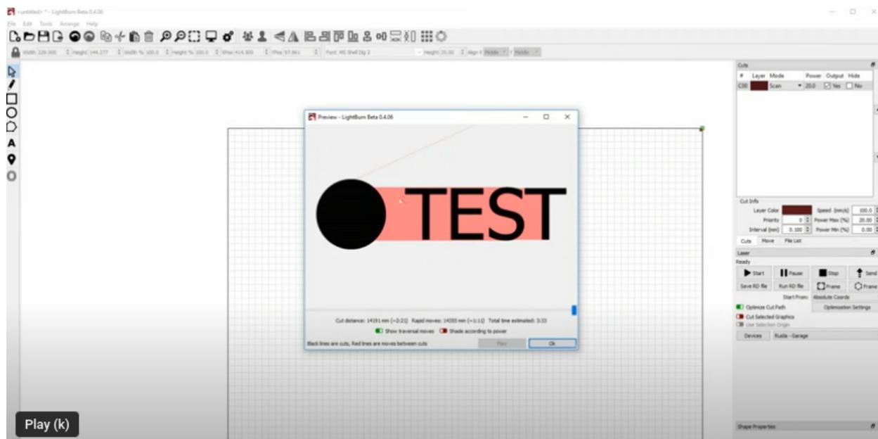
Example shape and text set to “fill” to create a vector engraving.
