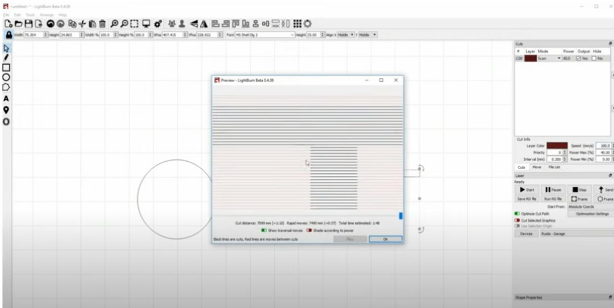
By default the interval is set to .1mm for an Ortur laser. Try changing it to .2mm, and you will find that the laser operation time is significantly reduced. Note that you will only be able to see this in the “preview” window, as interval does not get rendered in the main window.
