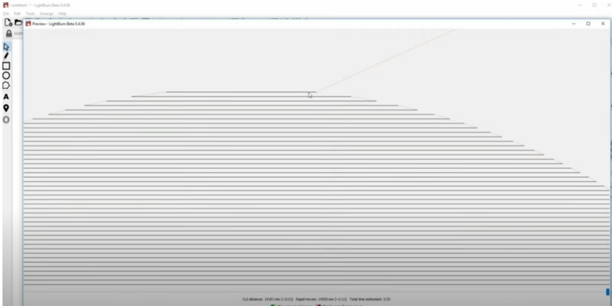
Once the pattern of movements has been generated, different “shades” of engrave can be achieved by setting the power level of the laser (a value between 0 and 100%) and the speed of the laser head, as controlled by the stepper motors. This speed will be dependent on the specifics of the machine.
